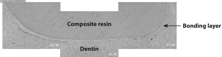
Fig. 1 Adaptation to cavity of Tokuyama Bond Force
